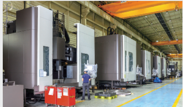
CNC Vertical Lathe Assembly Line
